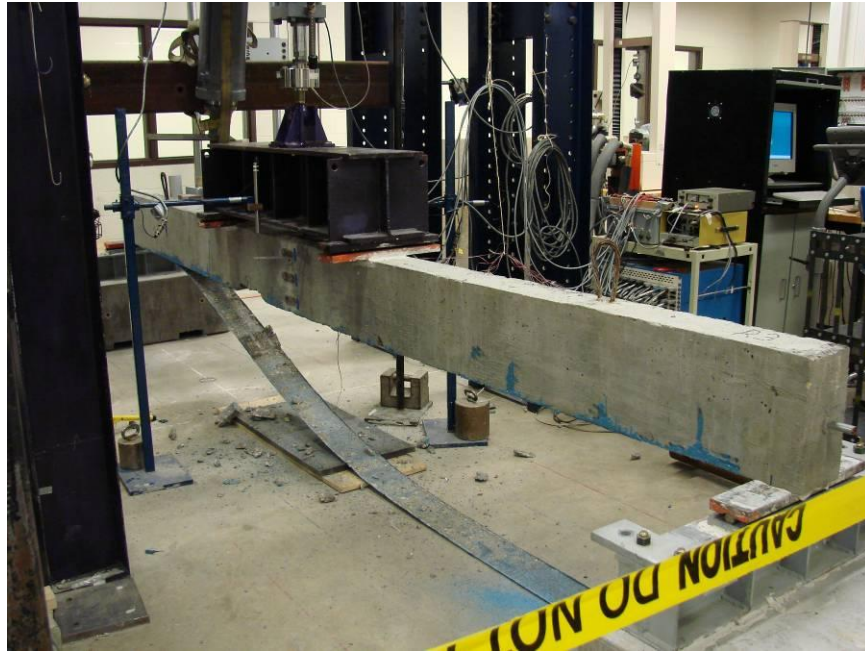
Figure 5.7 Beam R2 After Testing Showing Separation Failure of CFRP
