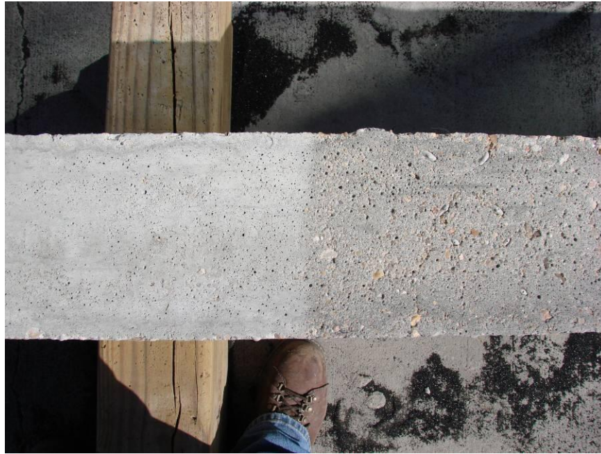
Figure 4.9 Comparison of Sanblasted (right) v. Non-Sandblasted Surface (left)
