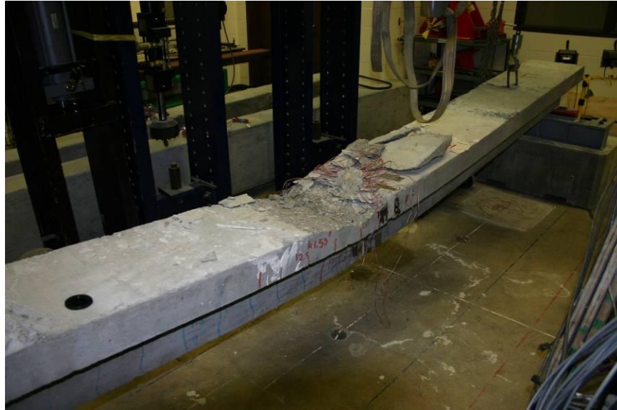
Figure 5.23 Beam T1 After Concrete Crushing Failure
