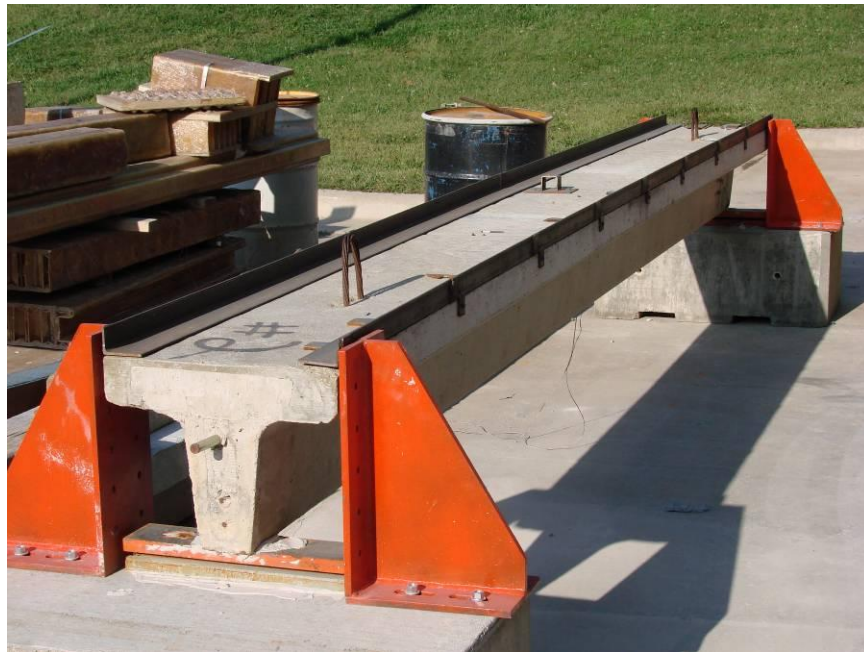
Figure 9.2 Setup of Bridge Girder Specimen
