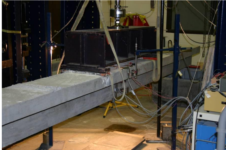
Figure 5.21 Control Beam T1 Before Testing
