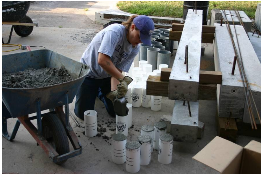
Figure 4.7 Casting of Concrete Cylinders
