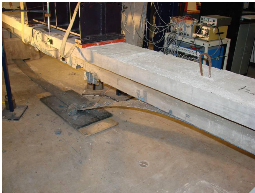
Figure 5.27 Failure of Beam T2 by Separation of Flexural CFRP
