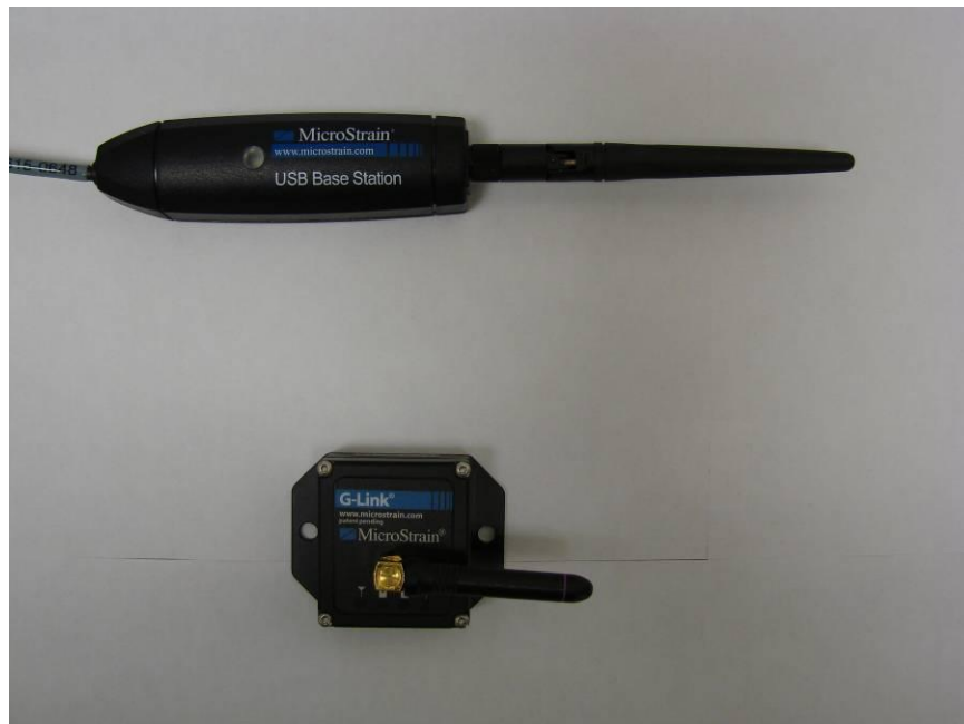
Figure 9.8 G-Link Wireless Accelerometer Node and Base Station
