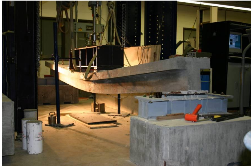
Figure 5.22 Beam T1 Just Prior to Failure
