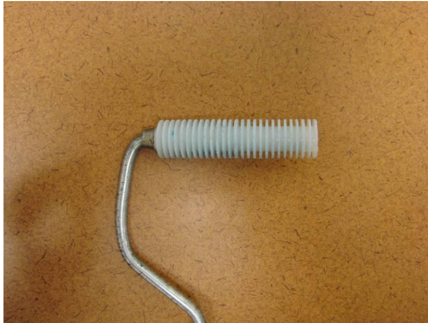
Figure 4.10 Roller Used for Application of CFRP
