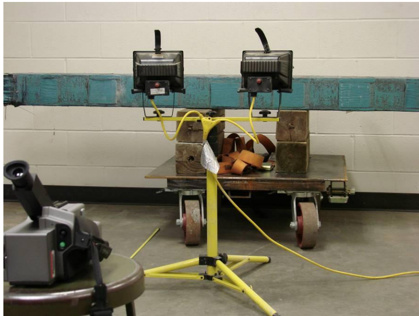
Figure 5.14 Infrared Thermography Setup
